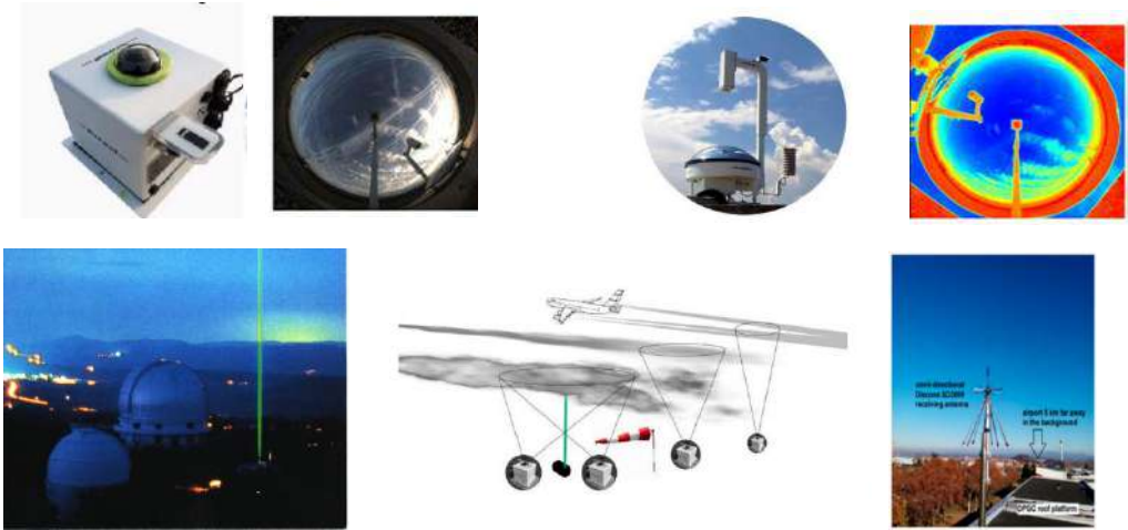
Fig. 3. upper-left: Sky Cam Vision™: Visible-range all-sky imager and visible contrails; upper-right: Sky InSight™: Thermal infrared all-sky imager and infrared view of contrails. The lower-left; view of the Lidar system operated by LATMOS in Observatory of Haute-Provence, France. The lower-middle figure is a schematic presentation of combination of camera with Lidar. Lower-right figure represents the schema of ADS-B system.
