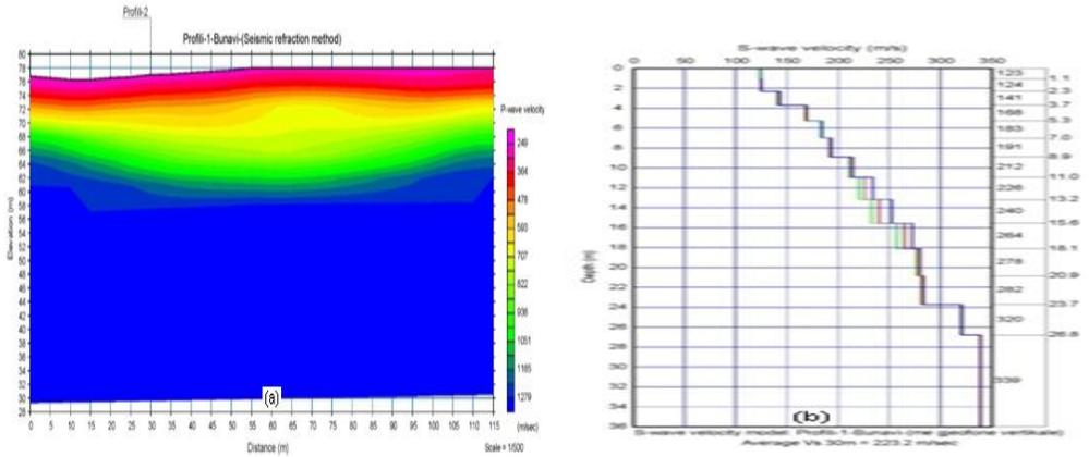
**Fig.7:** Seismic profile 1, Bunavi reservoir dam, Vlorë. (a)- 2D velocity model,  $V_p = f(h)$  according to refracted seismic waves.(b)- 1D velocity model,  $V_{S30} = f(h)$  according to surface seismic waves.
