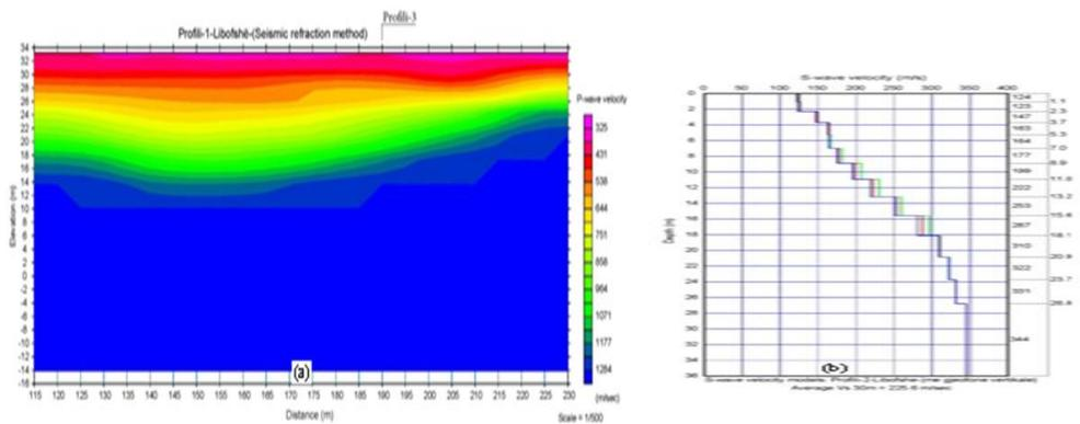
**Fig.12:** Seismic profile 1, Libofsha reservoir dam, Fieri. (a)- 2D velocity model,  $V_P = f(h)$  according to refracted seismic waves. (b)- 1D velocity model,  $V_{s30} = f(h)$  according to surface seismic waves.
