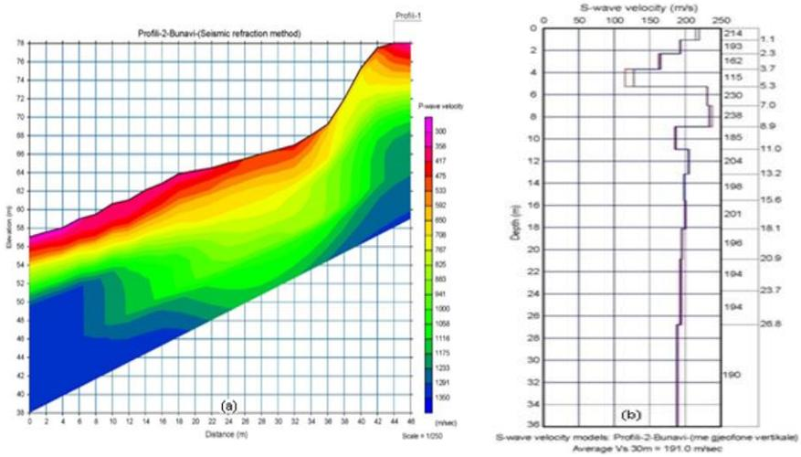
**Fig. 8:** Seismic profile 2, perpendicular to the Bunavi reservoir dam, Vlorë. (a)- 2D velocity model,  $V_p = f(h)$  according to refracted seismic waves. (b)- 1D velocity model,  $V_{S30} = f(h)$  according to surface seismic waves.
