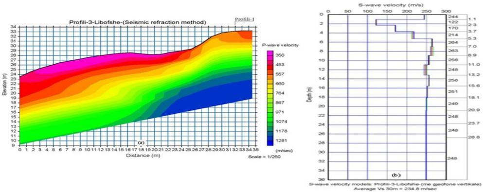
**Fig.13:** Seismic profile 3, Libofsha reservoir dam, Fieri.(a)- 2D velocity model,  $V_P = f(h)$  according to refracted seismic waves.(b)- 1D velocity model,  $V_{s30} = f(h)$  according to surface seismic waves.
