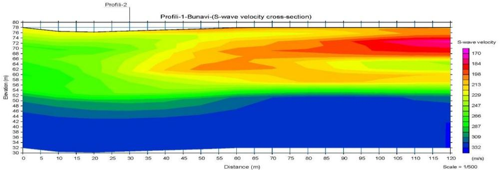
**Fig.9:** 2D velocity model according to surface seismic waves  $V_s = f(h)$ . Seismic profile 1, acquired with horizontal geophones.
