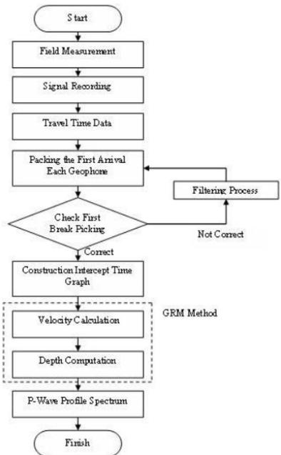
**Fig. 3:** Flow chart of refraction wave processing steps (SeisImager 2D).
