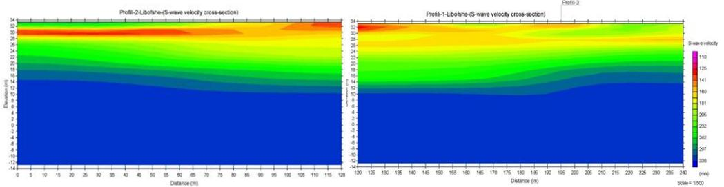
**Fig. 14:** Seismic profile (1+2), Libofsha reservoir dam, Fieri, recorded with horizontal geophones. 2D velocity model according to surface seismic waves  $V_s = f(h)$ . The soils that build the body of dam are inhomogenous.
