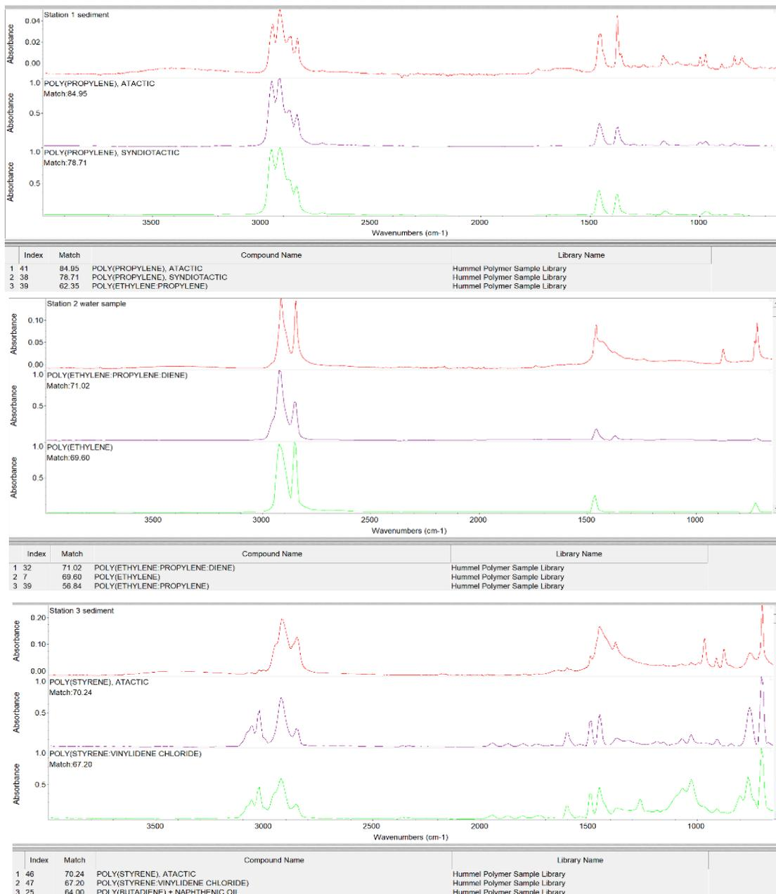
**Fig 3:** Examples of the FTIR spectra of the three microplastic particles found in the water and sediment samples, which were measured by micro-FTIR spectroscopy: upper panel polypropylene, second panel polyethylene, third panel polystyrene.
