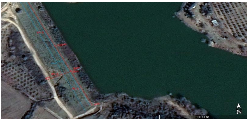
Fig. 10: Seismic profile placement in the Libofsha reservoir dam.
