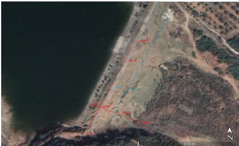
Fig.6: Placement of seismic profiles in the dam of the Bunavisa reservoir. Seismic profiles are in red. Electrometric profiles are in blue.
