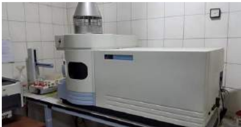
Fig. 2: Autosampler and Inductively Coupled Plasma ICP-OES, DV 2100, Perkin Elmer.
