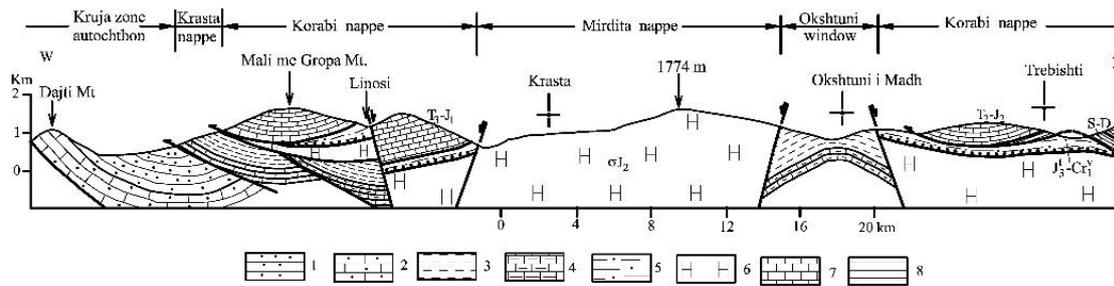
**Fig. 12:** Dajti Mountain-Trebishti Geological Section. Kruja Zone: 1- Upper Eocene-Lower Oligocene flysch, 2- Late Cretaceous neritic limestones. Krasta Zone: 3- Latest Cretaceous-Eocene flysch, 4- Late Cretaceous pelagic limestones. 5- Upper Jurassic-Lower Cretaceous marly flysch underlying Korabi nappes, 6- Middle Jurassic ultrabasic rocks, 7- Triassic-Jurassic limestones, 8- Silurian-Devonian schists.
