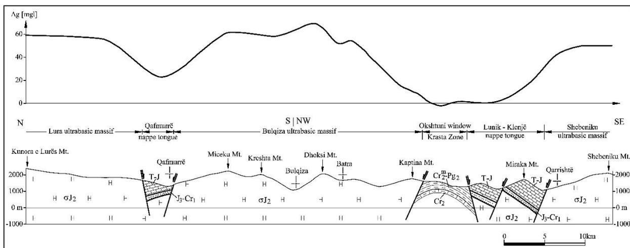
**Fig. 16:** Kunora e Lurës Mt.-Bulqiza-Shebeniku Mt. geological-geophysical section.
