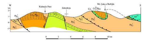
Fig. 2: W-E trending geological cross section Kulmaka Pass – Mt. Çuka e Bofnjes according to A-A line shown on Figure 1.
