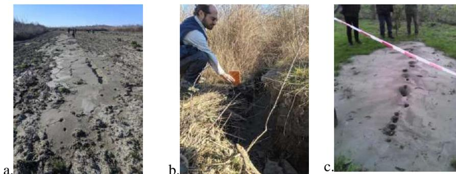
**Fig. 3.** a. Part of the southern branches of the lateral spreading near the river estuary. b. Vertical displacement of up to 15 cm was evident in certain places along the crack. c. Detail of sand ejecta along a crack in the area.
