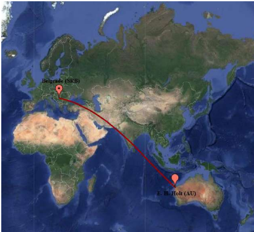
Fig.1: Propagation path NWC along GCP (red line), as transmitted from E. H. Holt (AU) towards Belgrade (SRB)
